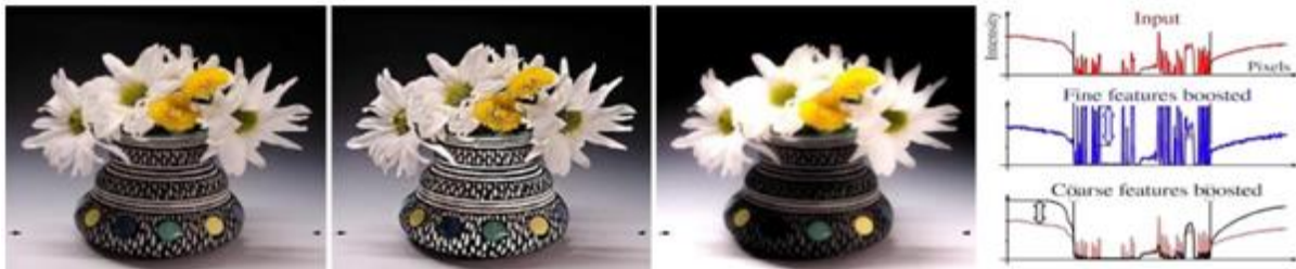
Figure 1: (a) allowing detail to be extracted based on spatial scale rather than contrast and preserves edges. (b) Boosting of fine scale features ;thus increasing contrast(c) Boosting of coarse scale contrast ;suppressing fine features ;thus reducing contrast of the pattern and increasing the contrast of the vase with background. (d) Scanline plots
